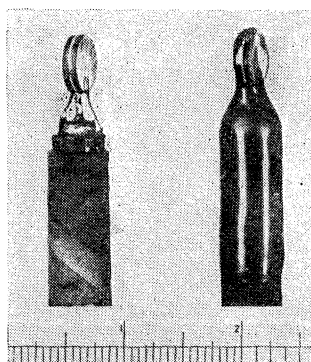
FIGURE 1. Piezo-electric gauge before application of rubberoid wax and natural latex. Also after completion of curing process.
